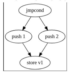
The value that is popped by the store v1 instruction has two possible values, and therefore two different data sources. In Echo, this would be encoded as a single DataDependency<TContents> with two possible data sources push 1 and push 2. The resulting data flow graph would therefore look something like the picture below:
