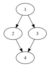
Dominator analysis give structure to CFGs, and can be very useful in static analysis to detect various constructs in a CFG such as loops, and reveal the importance of various nodes in terms of control flow.
